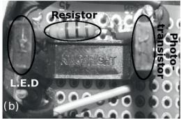
Fig. 3. (a) The experimental setup, with the metronomes placed on the platform and the wiring that carries information on the metronomes' phases. (b) One of the light-gates (Kingbright KTIR 0611 S), composed of an infrared LED and a photo-transistor.
