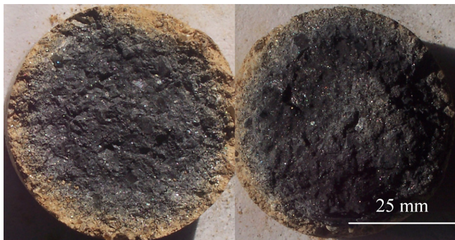
Fig. 11. Oxidation tests at 1200 °C for 3 h in air of MgO–C samples coked at 1000 °C in air and sealed by carbon in an alumina crucible, left TiO 2 -additions, right TiO 2 /Al-additions.
