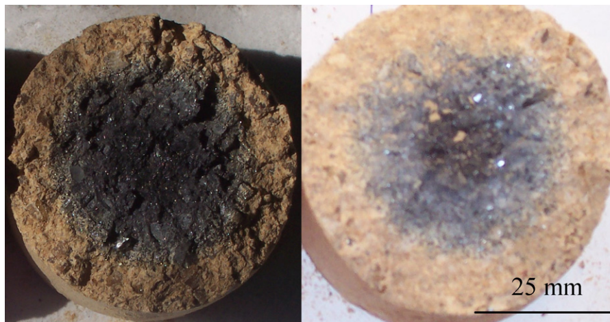
Fig. 10. Oxidation tests at 1200 ^{\circ} C for 3 h in air of MgO–C samples coked at 1000 ^{\circ} C in air and sealed by carbon in an alumina crucible, left with Al-additions, right no Al-additions.
